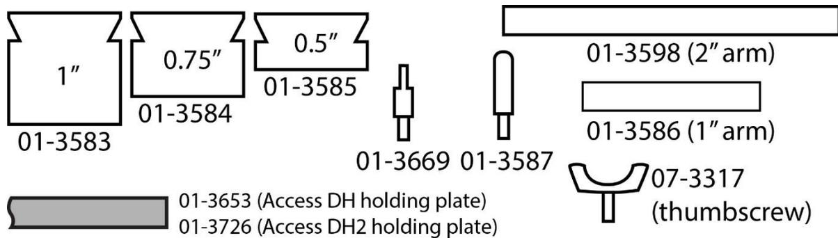
The kits pieces can be used to create a "Post Stack" which serves as an anchor support from the board edge, an adjustable "Rotating Stack" that supports the PCB from the board edge, a "Support Stack" which supports the PCB from underneath and a "Plate Stack" which uses a secondary holding plate. Use the diagrams shown on the following pages of this document to create stacks used with the Top, Middle, Bottom and Base slots of the Prober.
