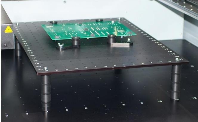
mounting of PCBs at a higher level. The plate is mounted on four Post Stacks and then additional spacers are added on top of the holding plate to secure the PCB in place. This method adds an additional degree of rigidity to the mounted board. The holding plate is 0.25" thick so the spacer sizes need to be adjusted to make up for the added height. The diagrams on the following pages showing the spacer Stack combinations include drawings using the additional holding plate
