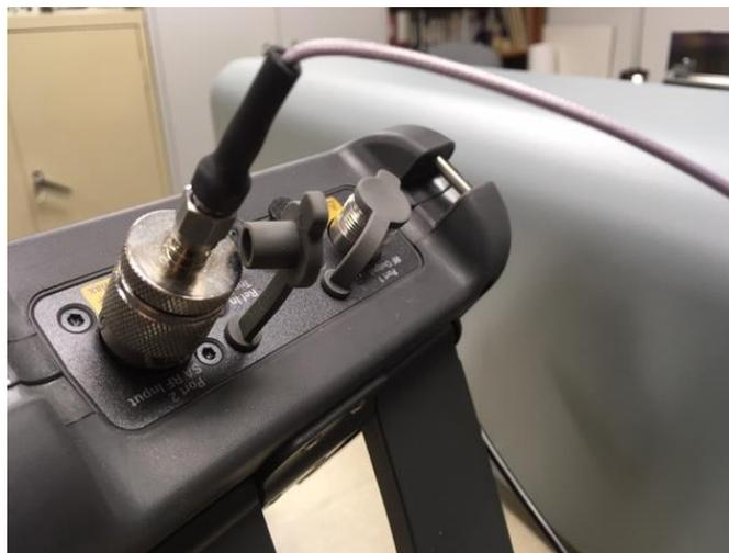
Connect the other end of the RF coax cable to the connector on the left rear panel of the Access RF prober.
